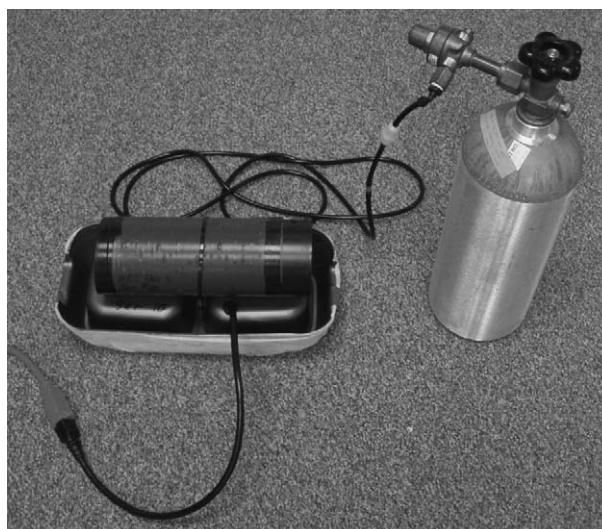
Fig. 1. Bedbug trap on the floor. The trap was plugged into an electrical outlet and the amount of CO 2 released from the cylinder was regulated by the attached regulator and orifice.
